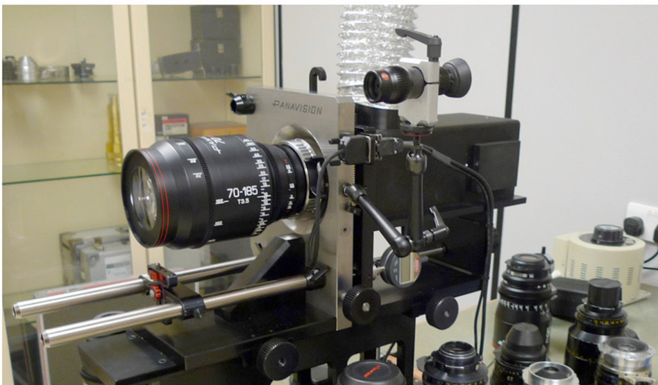
Hooked 7mm glass "plug" inserted behind Primo 70 lens on PV projector system
